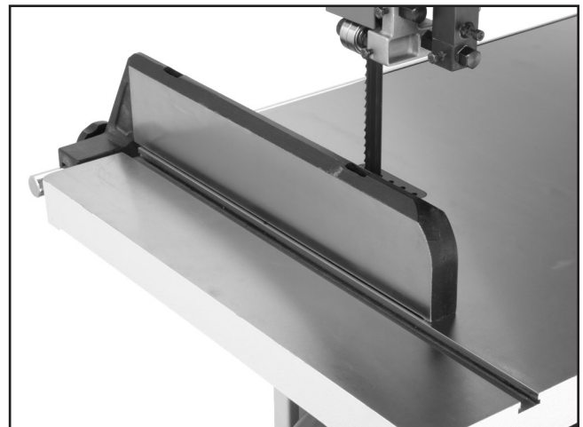
Figure 7. Example of fence square with miter slot.
